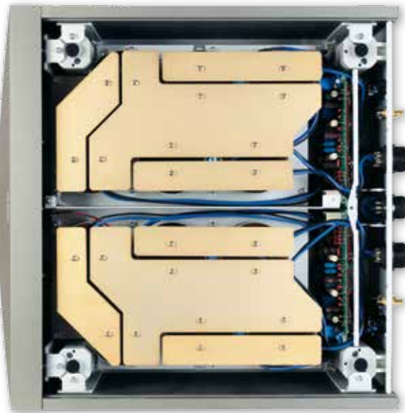
ABOVE: Gold-anodised plates inside the GM equaliser connect the six huge electrolytics feeding each side of the fully discrete, fully balanced filter and output stage [far right]
