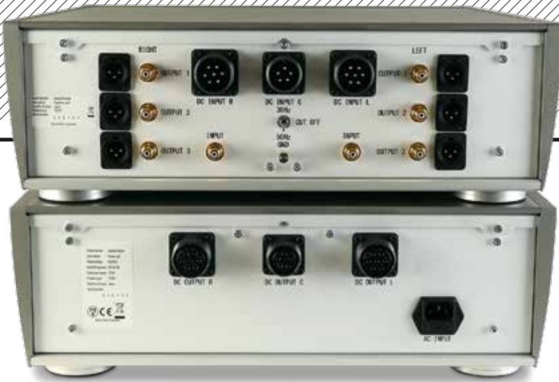
ABOVE: Rear view of the PSU [bottom] and equaliser [top]. The pick-up’s internal LEDs are powered via the R– and L– pins while the output is returned via R+ and L+, all via the ‘Input’ RCAs. Three eq’d line outs, on RCAs and balanced XLRs, offer three bass roll-offs from two different – 30Hz and 50Hz – turnover freqs. [see Graph 1, opposite]
